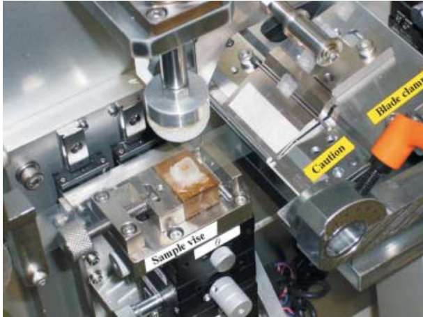
Fig. 4. Photograph of the main apparatus of the adhesive-film mediated automatic microtome (AFMA microtome). The blade on the holder (right) travels to the paraffin block (middle) to cut it. The stamping pad (upper) goes down to push the HistoFilm to the block to glue them together.
