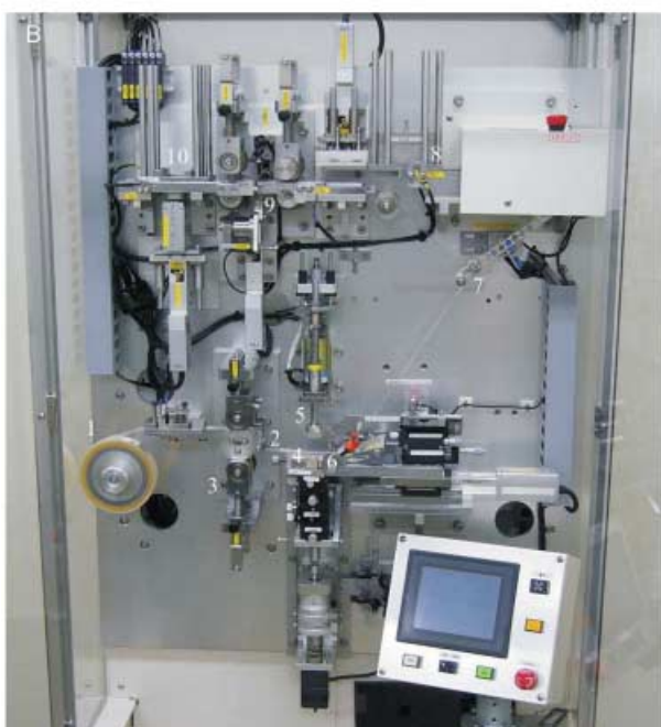
Fig. 2. Adhesive-film mediated automatic microtome (AFMA microtome). (A) Schematic illustration of the film machinery of the AFMA microtome. The HistoFilm (2) from the HistoFilm roll (1), after peeling off the protective film (3), is glued to the surface of a paraffin block (4) by a stamping pad (5), then the block is cut with the blade (6) just under the film to make a section attached to the film. A section-on-film goes up to the site where a plastic frame (8) is put on the film automatically and this is cut (9) to make a film slide (10), which looks like a glass slide. The tension roller (7) is important to ensure that the film is suitable for sectioning and also works as a tension sensor. If it detects abnormal tension, the machine can stop for safety. (B) A photograph of the AFMA microtome. The numbers in (B) correspond to ones shown in Figure 2A.
